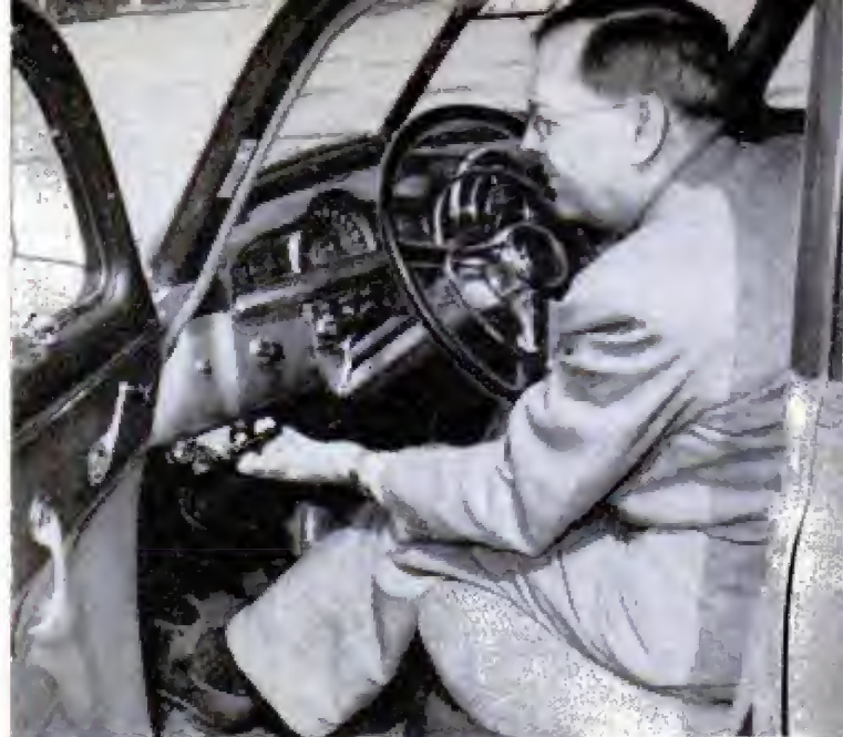
Hand-brake lever is mounted on swivel bracket for ease of operation. Clymer liked red warning light
